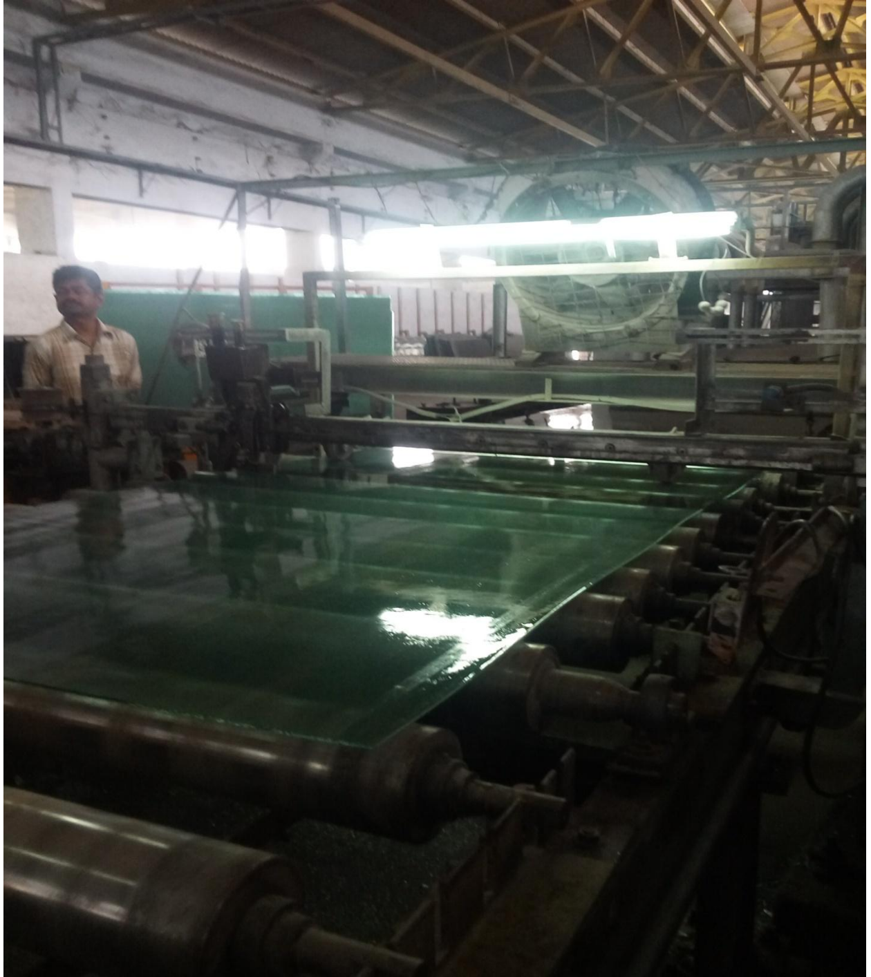
THE OUTCOMING OF PREPARED GLASS FROM FURNCE (COOLED GLASS)
